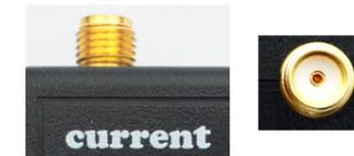
The signal output delivers the measured and processed current which is represented by a voltage value (i.e. 10mA per V). The output can be connected with an SMA cable to a voltage measurement device (high impedance input), typically an oscilloscope.
